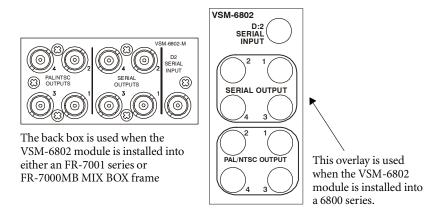
Figure 12-2. Back Module and Overlay
